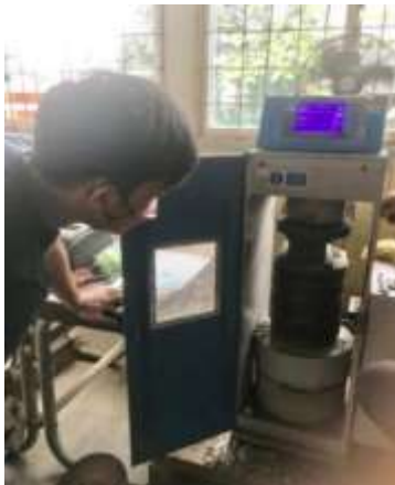
(a) Pengujian kuat tekan paving block
