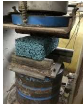
(b) Pengujian kuat lentur paving block
