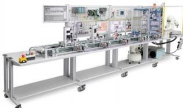
Gambar 1. *Industrial Mechatronics System* (IMS)
